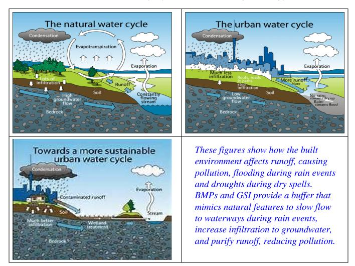
These features include rain gardens, bio-swales, vegetated planting strips, green roofs, tree pits, constructed wetlands, and other green features intended to mimic natural features. In addition to providing improved stormwater management, these features provide aesthetic benefits for the community, increased habitat areas for wildlife, improve air quality, and enhance water quality.
